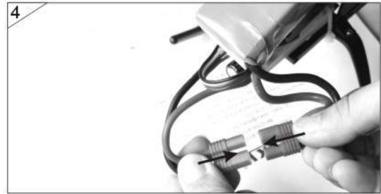
Connect helicopter's electricity
