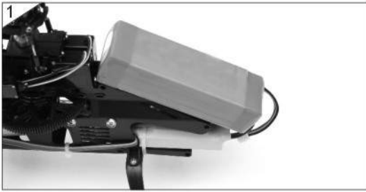
Insert the battery to the battery notch
