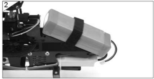
Fix the battery's position with the bandage
